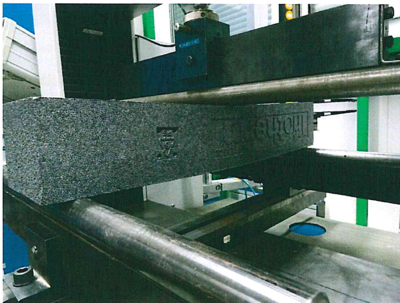
Fig. 7: Test setup bending behaviour (exemplary representation)
